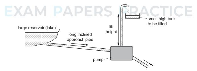
In one such pump the long approach pipe holds 500 kg of water. A valve shuts when the speed of this water reaches 2.0 m s<sup>-1</sup> and the kinetic energy of this water is used to lift a small quantity of water by a height of 15 m.
