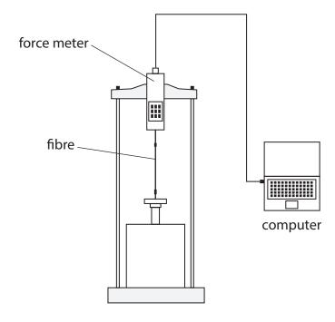
The apparatus shows a force meter that pulls on the attached fibre. The force needed to break the fibre is recorded on the computer.
