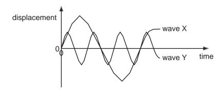
Wave X has amplitude 8 cm and frequency 100 Hz.
