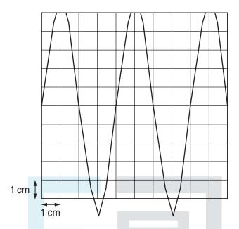
The oscilloscope time-base setting is 0.5 ms cm<sup>-1</sup> and the Y-plate sensitivity is 2 V cm<sup>-1</sup>.
