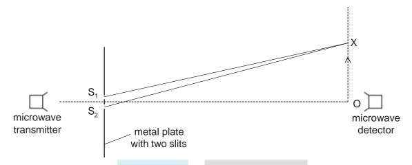
The detector is moved from point O in the direction of the arrow. The signal detected decreases until the detector reaches point X, and then starts to increase again as the detector moves beyond X.
