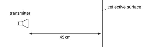
The emitted waves have a frequency of 1.00 GHz. A stationary wave is produced with a node at the transmitter and a node at the surface.
