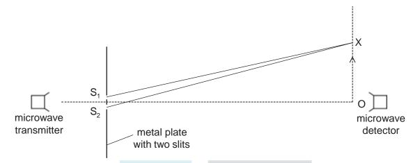
The detector is moved from point O in the direction of the arrow. The signal detected decreases until the detector reaches point X, and then starts to increase again as the detector moves beyond X.
