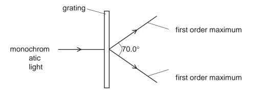
The spacing of the slits in the grating is  $1.00 \times 10^{-6}$  m. The angle between the first order diffraction maxima is 70.0°.
