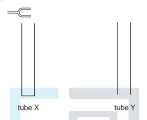
The tubes are identical except tube X is closed at its lower end while tube Y is open at its lower end. Both tubes have open upper ends.
