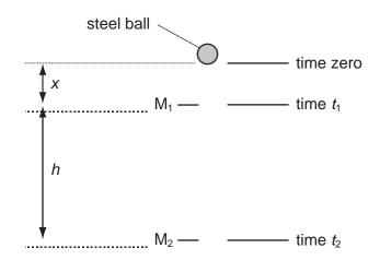
A steel ball is released at time zero from a point a distance x above M<sub>1</sub>. The ball reaches M<sub>1</sub> at time  $t_1$  and reaches M<sub>2</sub> at time  $t_2$ . The acceleration of the ball is constant.
