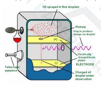
In Millikan's Oil Drop Experiment oil is sprayed into a chamber before passing between metal plates where the electric and gravitational forces are compared
