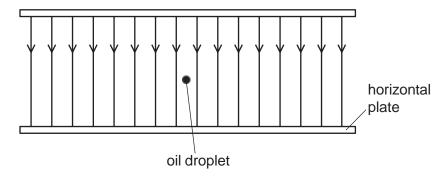
The weight of the droplet is exactly balanced by the electrical force on the droplet.
