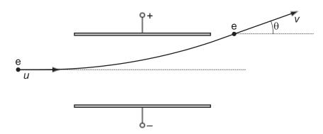
While in the electric field, its direction changes by  $\theta$  and it emerges with a velocity v.
