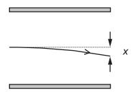
The vertical deflection x is measured at the right-hand edge of the plates.
