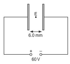
What is the electric field strength at E, a point midway between the plates?
