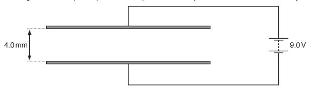
What is the electric field strength between the plates?
