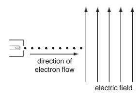
An electron gun injects a beam of electrons horizontally into the field.
