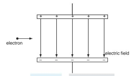
What are the horizontal and vertical components of the motion of this electron when it is in the field?
