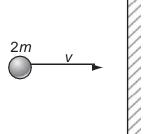
The particle rebounds along the same path after colliding with the wall. The collision is inelastic.
