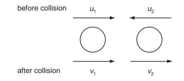
Which equation is correct if the collision is perfectly elastic?
