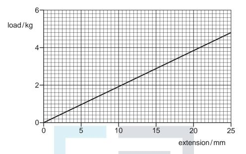
How much work is done on the wire to increase the extension from 10mm to 20mm?
