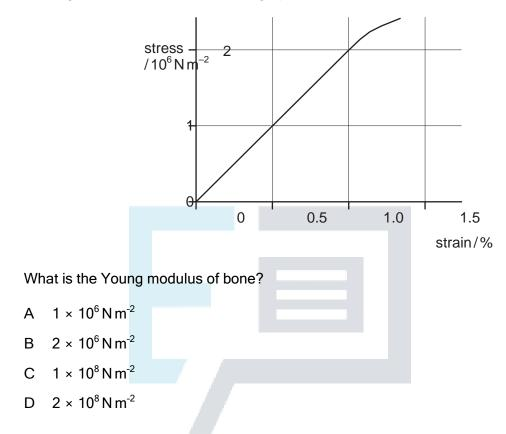
54. The diagram shows the stress-strain graph for bone.
