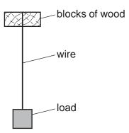
By how much would a wire of the same material, but of diameter 2*D* and length 3*L*, extend when the same load is applied?
