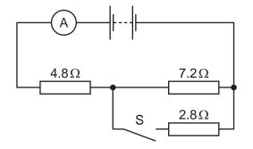
When S is open, the reading on the ammeter is 250 mA.
