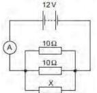
The battery has e.m.f. 12 V and negligible internal resistance. The ammeter reading is 3.2 A. What is the resistance of X?
