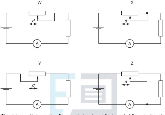
The distance *d* between the sliding contact and a particular end of the potentiometer is varied. The current measured is then plotted against the distance *d*.
