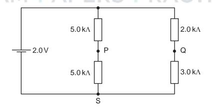
$V_1$  is the potential difference between S and P.  $V_2$  is the potential difference between S and Q. What is the value of  $V_1 - V_2$ ?
