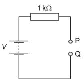
A student attempts to measure the potential difference (p.d.) between points P and Q using two voltmeters, one at a time. The first voltmeter has a resistance of  $1 k\Omega$  and the second voltmeter has a resistance of  $1 M\Omega$ .
