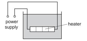
The heater has a resistance of 3.0  $\Omega$ . The power supply has an e.m.f. of 12 V and an internal resistance of 1.0  $\Omega$ .
