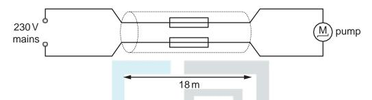
The performance of the pump is acceptable if the potential difference (p.d.) across it is at least218 V. The current through it is then 0.83 A.
