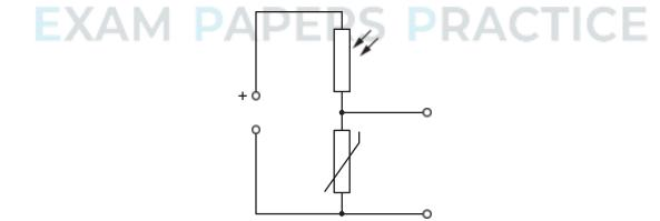
Under which set of conditions will the potential difference across the thermistor have the greatest value?
