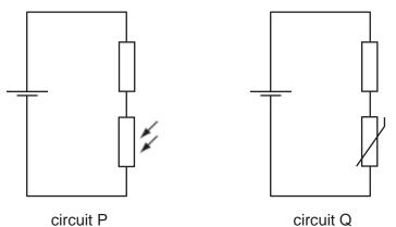
How does the potential difference across the fixed resistor in each circuit change when both the brightness of the light on the light-dependent resistor and the temperature of the thermistor are increased?
