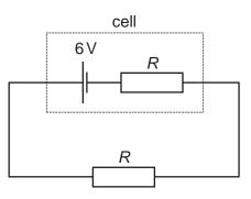
Power *P* is dissipated by the external resistor.
