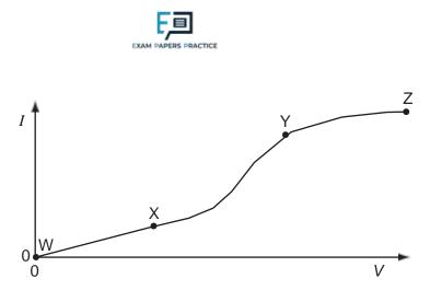
In which ways does the resistance of the component vary within each of the three sections?
