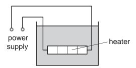
The heater has a resistance of 3.0  $\Omega$ . The power supply has an e.m.f. of 12 V and an internal resistance of 1.0  $\Omega$ .
