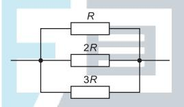
Using I to represent the current through the resistor of resistance R, which row represents the relationships between the currents through the resistors?
