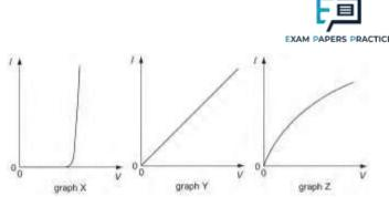
The components are a metal wire at constant temperature, a semiconductor diode and a filament lamp. Which row of the table correctly identifies these graphs?
