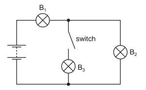
Initially the switch is closed. The switch is then opened and lamp  $B_3$  goes out.
