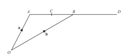
A and B have position vectors  $\mathbf{a}$  and  $\mathbf{b}$  relative to the origin O. C is the midpoint of AB and B is the midpoint of AD.
