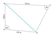
A fence is built connecting points B and D to split the paddock into two.
