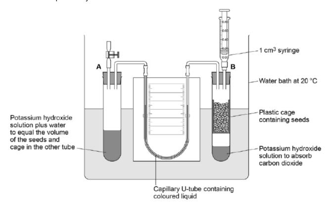
(a) For the first 10 minutes, the tap attached to tube **A** was left open and the syringe from tube **B** was removed.
