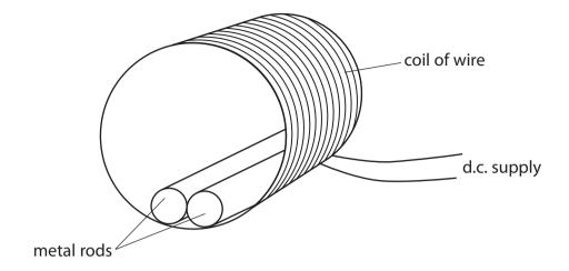
(a) When a direct current is supplied to the coil, a magnetic field forms and the metal rods move apart.
