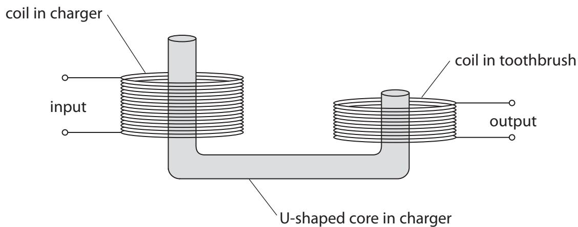
This arrangement of core and coils acts as a transformer that reduces voltage.
