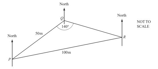
The diagram shows three points P, Q and R on horizontal ground.
