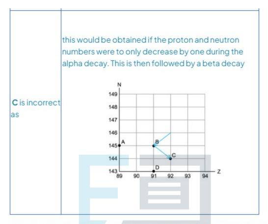
To be able to answer these questions correctly, you need to recall that alpha decay is the emission of two neutrons and two protons (a helium-4 nucleus) and that beta decay involves a neutron changing into a proton. This is a diagonal right on the diagram above, but watch out - the axes may not always be this way round! It's better to understand what's going on in each decay as opposed to memorising the paths on an N-Z graph.
