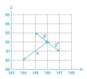
Alternatively, you could write out an equation to determine the N and Z values and then find the correct point on the graph
