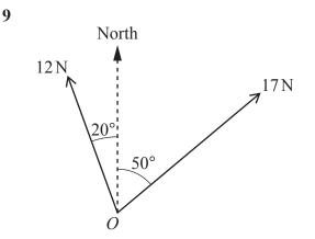
Two horizontal forces of magnitudes 17 N and 12 N act at a point *O* along bearings of  $050^{\circ}$  and  $340^{\circ}$  respectively (see diagram).
