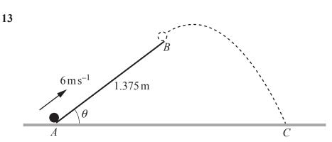
The points *A* and *B* are the lower and upper ends, respectively, of a line of greatest slope on a plane inclined at an angle  $\theta$  to the horizontal, where  $\sin \theta = 0.6$  and AB = 1.375 m (see diagram).
