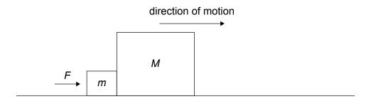
What is the force that the block of mass M is exerting on the block of mass m?
