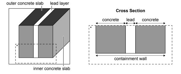
The width of a concrete slab is modelled by a normal distribution with mean  $350 \,\mathrm{mm}$  and standard deviation  $10 \,\mathrm{mm}$ .
