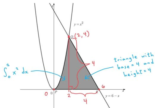
Point  $P$  is the point of intersection of the curve  $y = x^2$  with the  $x$ -axis. Point  $Q$  is the point of intersection of the curve  $y = x^2$  with the line  $y = 6 - x$  for which  $x > 0$ . Point  $R$  is the point of intersection of the line  $y = 6 - x$  with the  $x$ -axis.
