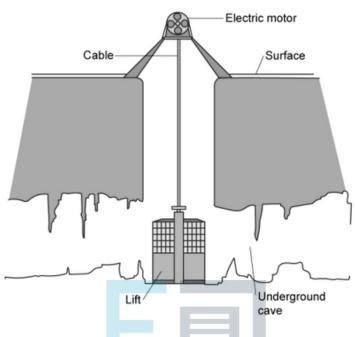
Each caver has a mass of 50 kg and the lift has a mass of 340 kg. The winch raises the lift through a vertical height of 2 km in 3 minutes.
