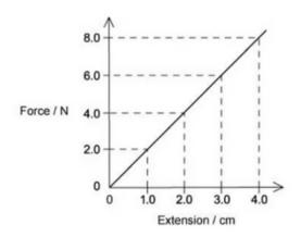
What is the work done on the wire to increase the extension from 4.0 to 5.0 cm?
