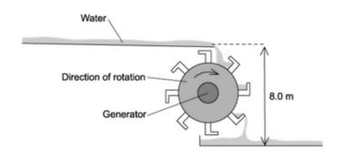
Ignore any changes in the kinetic energy of the water. What is the efficiency of the system?
