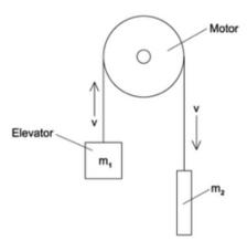
What rate does the motor provide energy to the system when the elevator is rising at a steady speed v m s<sup>-1</sup>?
