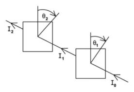
Which sheet must be rotated and by what angle so that light of intensity  $\frac{1}{4}$  I  $_0$  emerges from the second sheet?
