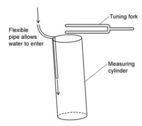
A tuning fork is made to oscillate and held over the open end. A resonant frequency is heard early on in the experiment and then again after a further  $5.5 \times 10^{-3}$  m<sup>3</sup> of water has run into the cylinder.
