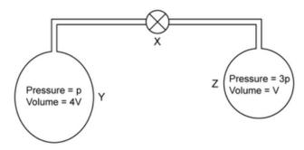
Initially the valve X is closed and gas bottle Y has a volume 4V and contains Hydrogen at a pressure p. Gas bottle Z has a volume V and contains Hydrogen at a pressure of 3p. Y and Z are initially at the same temperature.
