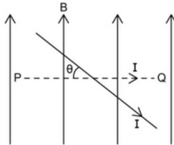
The current-carrying wire is then rotated clockwise through an angle  $\theta$  about an axis perpendicular to the plane of the image.
