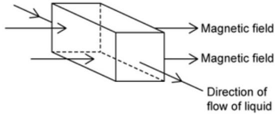
An electric field is set up in the pipe
