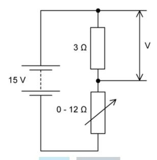
The power supply has an emf of 15 V and negligible internal resistance.
