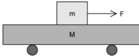
A horizontal force  $F$  acts on the block causing it to slide over the trolley. What is the acceleration of the trolley?
