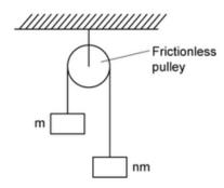
What is the acceleration of the masses a and the tension in the string T?
