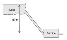
The mass flow rate of the water is 3000 kg min<sup>-1</sup>. The turbine has an efficiency of 60%. Acceleration due to free fall is 10 m  $s^{-2}$ .
