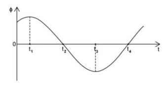
Determine the times when the magnitude of the induced emf measured across the ends of the coil is at a minimum.
