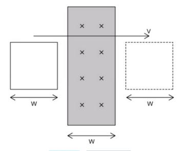
From the point where the coil enters the field until the point where it leaves it, which description best fits the direction of the current induced in the coil?
