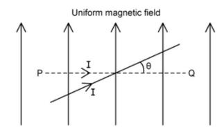
The current-carrying wire is then rotated anti-clockwise through an angle  $\theta$  about an axis perpendicular to the plane of the diagram.
