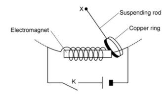
An electromagnet is set up so that the ring can pass over it as it swings. The ring is then set into oscillation at time t = 0, with switch K open. It completes two full oscillations, at which point the switch K is closed at time  $t = t_0$
