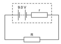
A charge of 240 C through the resistor in two minutes. The power dissipated in the resistor as a result is 1440 J. What is the internal resistance *r* of the battery?
