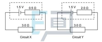
Which row in the table below correctly describes the potential difference across and power dissipated by the 3  $\Omega$  resistor?
