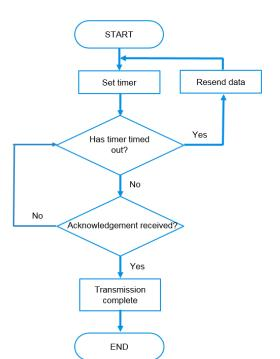
A ARQ flowchart shows a system of transferring data.
