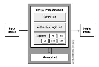
Von Neumann architecture design consists of a Control Unit, Arithmetic and Logic Unit (ALU), Memory Unit, Registers, and Inputs/Outputs.
