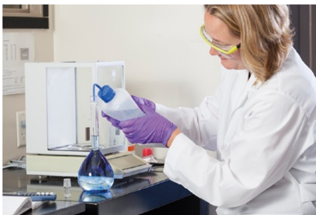
Figure P2.2 Volumetric flasks are used to make up standard solutions of known concentration accurately.
