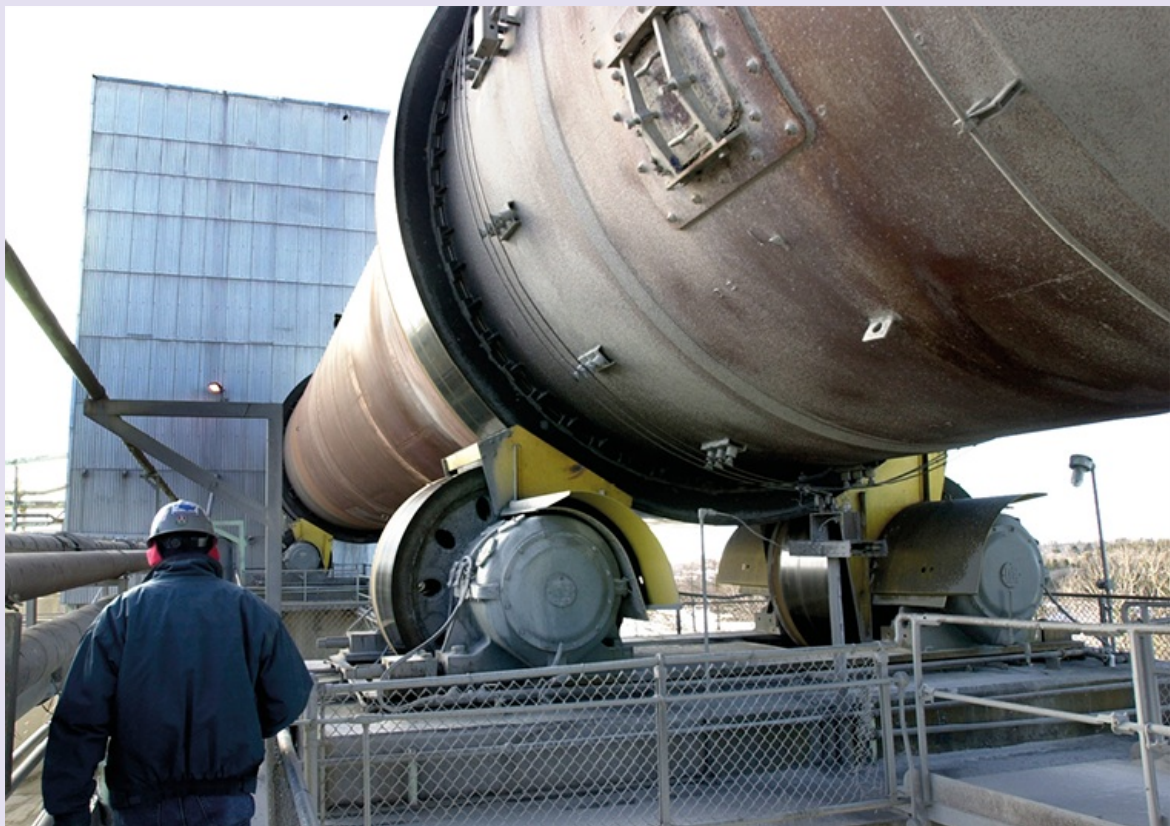
Figure 11.2: In a rotating lime kiln, calcium carbonate undergoes thermal decomposition to form calcium oxide and carbon dioxide.
