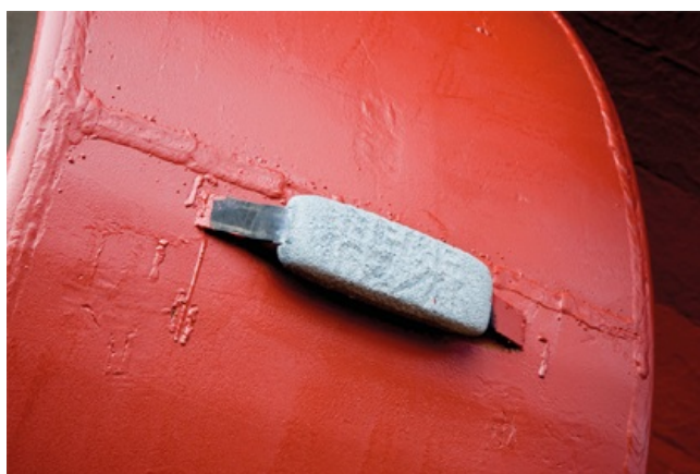
Figure 7.2: This is part of a ship's hull. It is made of iron protected by bars of magnesium metal. The magnesium atoms (oxidation number = 0) are oxidised to \text{Mg}^{2+} ions (oxidation number = +2) in preference to iron atoms changing to \text{Fe}^{3+} . This is called sacrificial protection .
