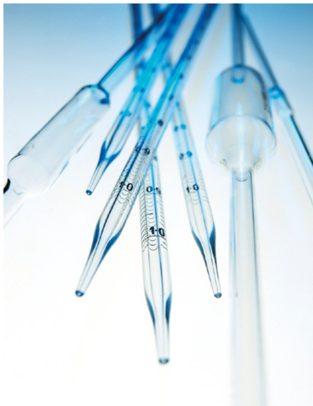
Figure P2.3 Volumetric and graduated pipettes are used to transfer accurate volumes of liquid. Volumetric pipettes give greater accuracy than graduated pipettes, due to the single line to measure to on the thin section above the bulge.
