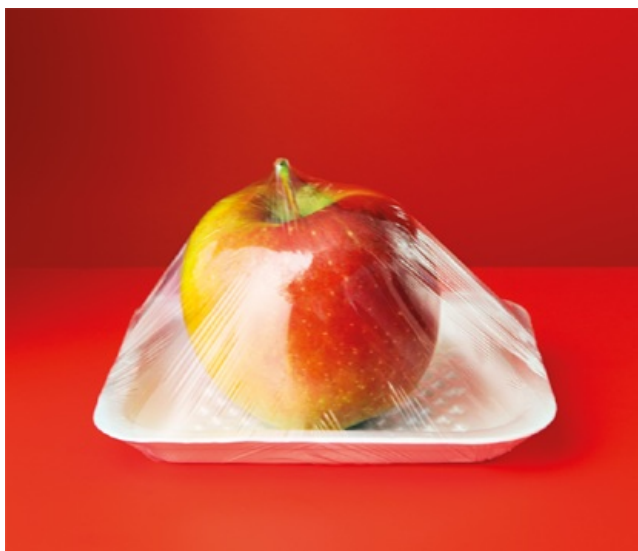
Figure 22.15: Addition polymers are produced using metallocene catalysts such as [(\text{C}_5\text{H}_5)_2\text{ZrCH}_3]^+ . The strength and puncture resistance of this polymer film have made it popular for food packaging.
