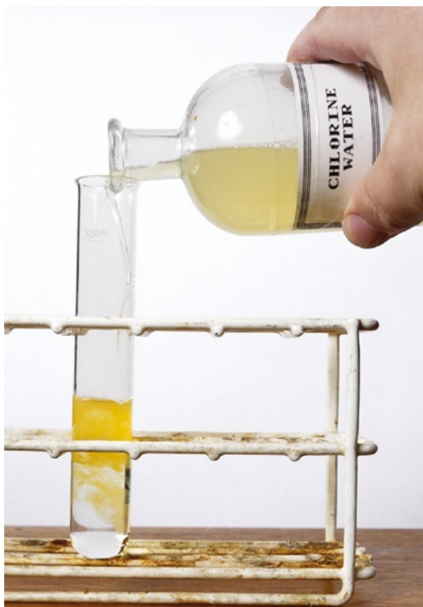
Figure 20.23: Aqueous chlorine displaces bromine from a solution of potassium bromide. We can use E^\ominus values to explain why a halogen higher in Group 17 displaces a halogen lower in the group from a solution of its halide ions.
