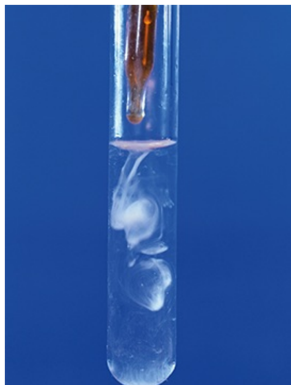
Figure 25.6: Bromine water is added to aqueous phenol from a dropper to form 2,4,6-tribromophenol.
