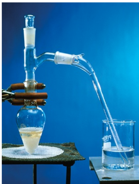
Figure 17.4: Bromoethane being distilled off following the reaction between ethanol and hydrogen bromide. The white solid visible in the pear-shaped flask is sodium bromide (crystals). The sodium bromide reacts with concentrated sulfuric or phosphoric(V) acid to make the hydrogen bromide needed for the reaction.
