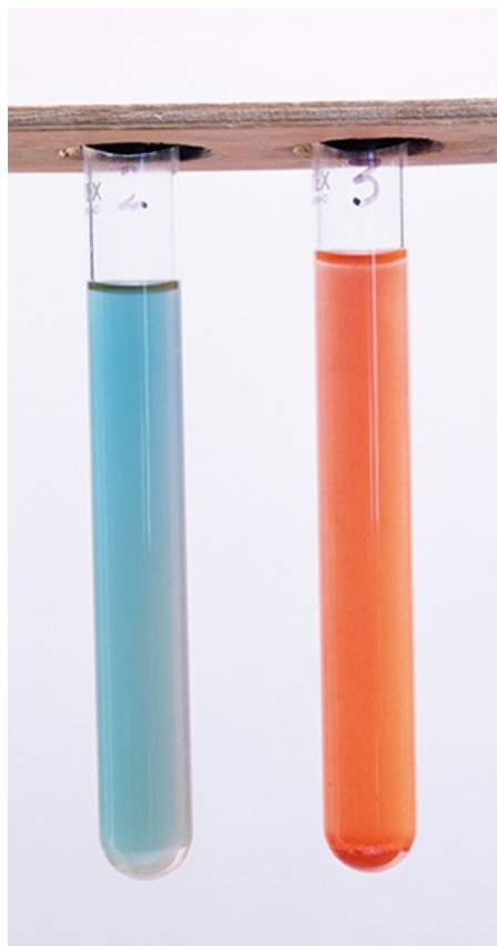
Figure 18.5: 'The 'before' and 'after' observations when Fehling's solution is warmed with an aldehyde, such as ethanal, \text{CH}_3\text{CHO} .
