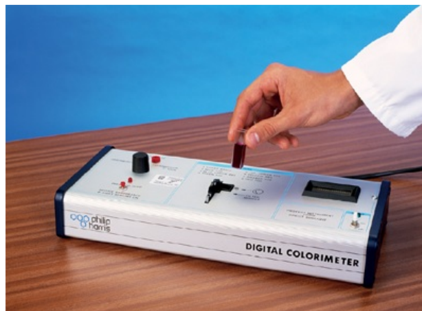
Figure 9.2: We can use a colorimeter to monitor the progress of a reaction. It measures the transmission of light through a 'cell' containing the reaction mixture. The less concentrated the colour of the reaction mixture, the more light is transmitted through the 'cell'.
