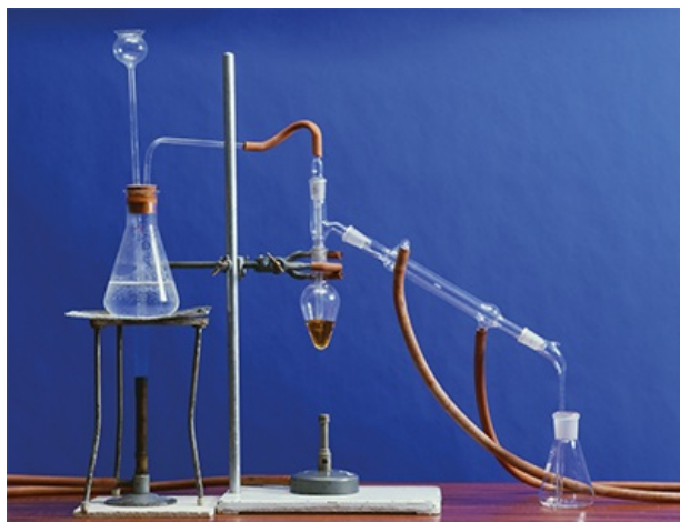
Figure 27.7: Steam generated in the conical flask is passed into the reaction mixture in the pear-shaped flask and phenylamine is distilled off and collected.
