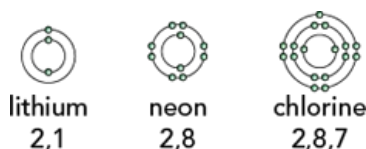
Figure 2.3: The simple electronic structures of lithium, neon and chlorine. The nuclei of the atoms are not shown.
