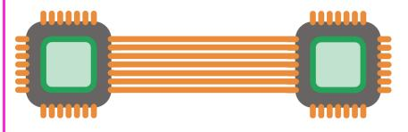
Each line within a parallel communication system will have very slightly different electrical properties, meaning that signals will take a very slightly different amount of time to travel across them. As a result, not all data sent at the same time will arrive at the
