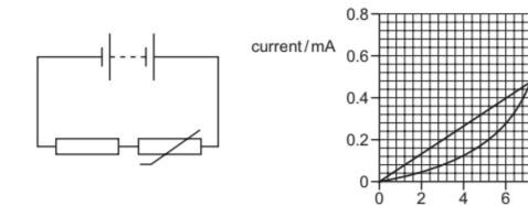
The battery has an e.m.f. of 12 V and negligible internal resistance.
