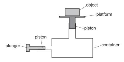
The plunger is slowly pushed 4.0 cm to the right. As a result, the object slowly moves upwards a distance 0.50 cm.
