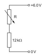
What is the resistance of the variable resistor R to give a potential difference of 1.0 V across the  $12 k\Omega$  resistor?
