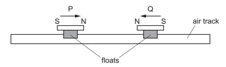
The two magnets slide towards each other along the air track and interact, without making contact.
