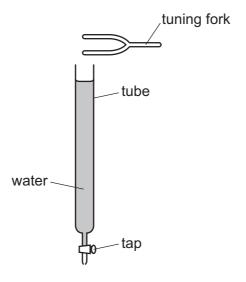
A louder sound is heard at intervals as the water runs out of the tube. The change in water level between louder sounds is 32 cm.
