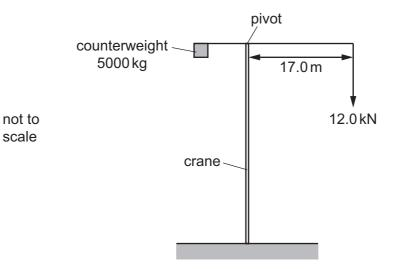
The counterweight has a mass of 5000 kg. The crane is required to lift a load of 12.0 kN and the horizontal distance from the pivot to the load is 17.0 m.
