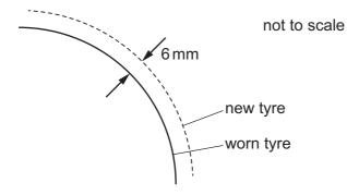
What is the error in the speed shown on the speedometer after this wear has taken place?
