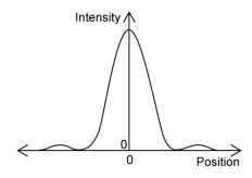
The width of the slit is increased. The original diffraction pattern is shown by the solid line.
