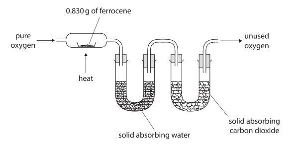
The hydrogen atoms from the sample react with oxygen to form water, which is absorbed in the first U-tube.
