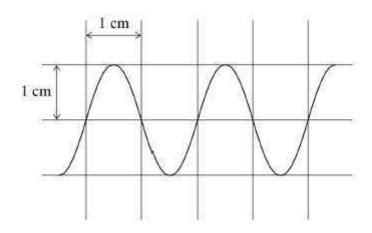
The time base setting is 5 ms cm<sup>-1</sup> and the Y-voltage gain is 10 V cm<sup>-1</sup>.
