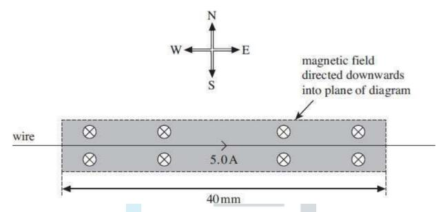
When a current of 5.0 A passes through the wire from west to east, a horizontal force acts on thewire. Which line, A to D, in the table gives the magnitude and direction of this force?
